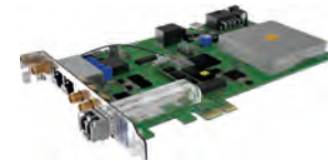
OSA 5400 TimeCard™ Half-size PCIe card, PTP grandmaster, NTP server, boundary/slave clock
