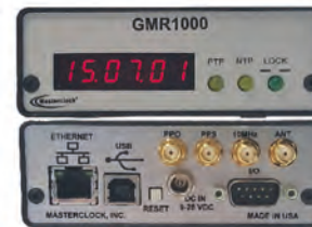
Masterclock GMR1000 NTP, PTP, IRIG-B, and SMPTE – synchronization optionally via OCXO, Rubidium, or GPS/GNSS.
